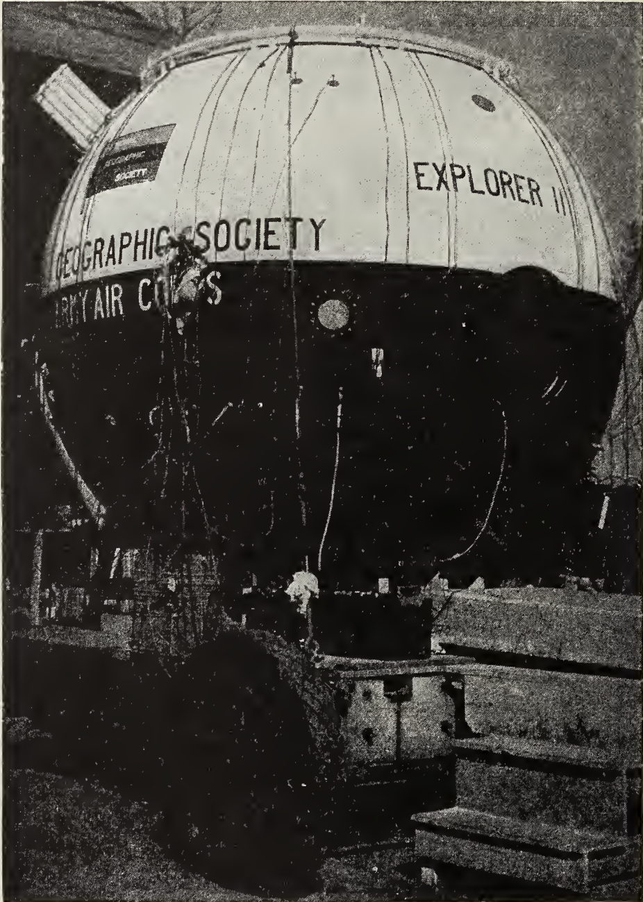
Fig. 28. Gondola of the balloon Explorer II
